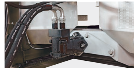
Central hydraulic drive (for RO-XL/RO-EDW/RO-EDW GEOspread)
