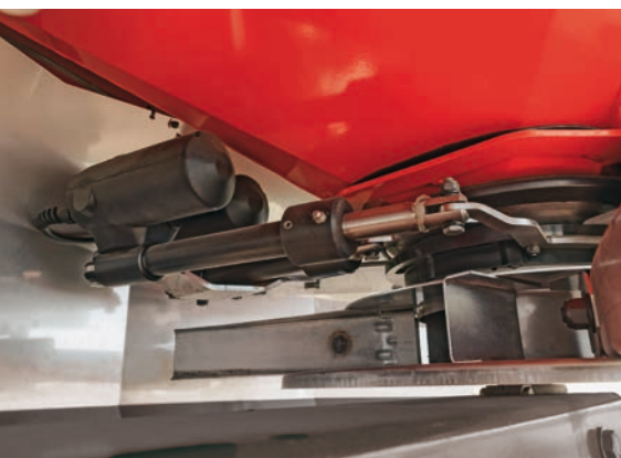
Two actuators on each dosing unit to control the discharge point and application rate
