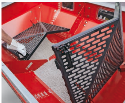
Grid locked in open position
