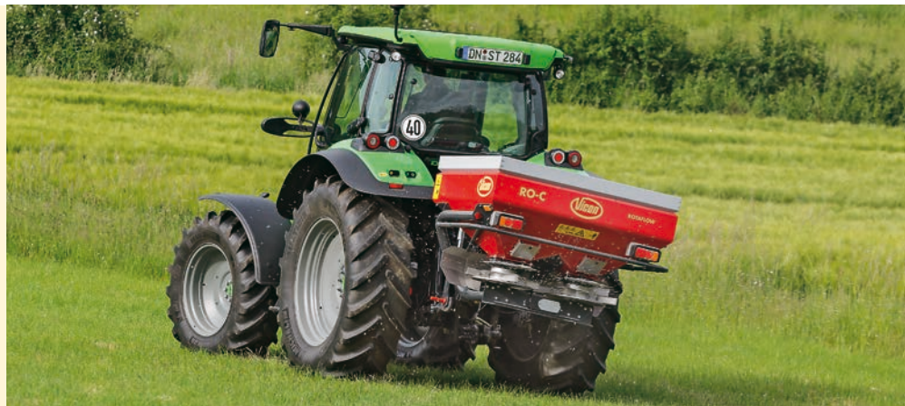
Border spreading from the tramline
