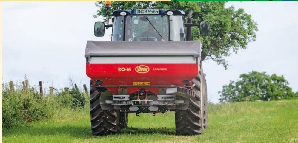
Border spreading using the border spreading plate (available as manual or hydraulic version)
